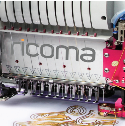
CORDING DEVICE Easily create an embroidery effect with the cording device, which lays cord on fabric and attaches the cord with transparent zigzag stitches.
