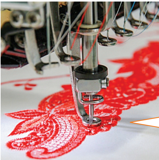
BORING DEVICE This device punctures holes into embroidered designs and encloses the raw edges with stitches to create a beautiful effect within minutes.
